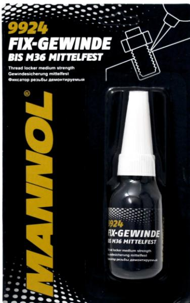
**GB** Mannol Fix-Gewinde bis M36 mittelfest prevents unscrewing the threaded metal connections with a step of cutting up to M36. Withstands vibration, applicable to engines, transmissions, gear boxes. Fills the interior surface of the thread. Prevents leakage of oil, water, air and corrosion. Withstands torque at M10 to 20 Nm. Operating temperature of -55 °C to +150 °C.
